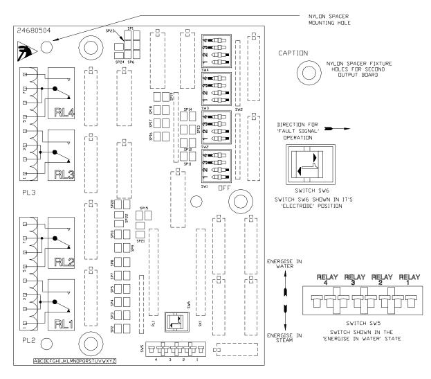
Figure 3a.1 - View of relay output board showing switch positions and output pin details
